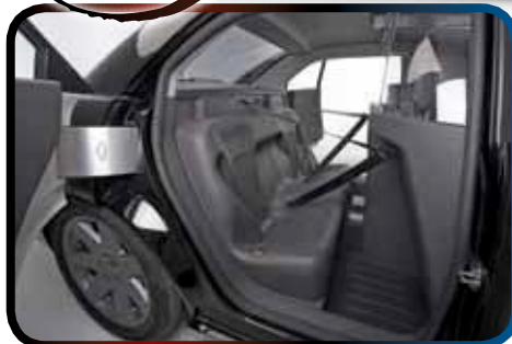
The prisoner seat has easy-to-use seat belts and the whole area is sealed off from the front compartment so prisoner-yuck can't sneak forward. There are drain holes in the floor to make hosing it out a breeze.
